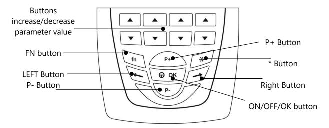
ON/OFF/OK button...... Confirms the selection, starts and pauses the treatment. Pressed for 3 seconds, it allows switching on and off.
