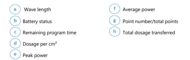
By keeping the \* key pressed, you go to the screen-page that usually characterizes a laser therapy protocol. The following screen-page will appear with the specific parameters of the program being executed:
