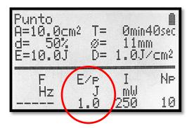
Also in this case, by acting on the four Up and Down buttons, it is possible to modify the frequency (if the pulsed emission mode has been chosen), the program duration, the power intensity and the size of the area to be treated, combining them in order to obtain the desired protocol. By pressing the \* key, the parameter "D" (Power density) in J / cm<sup>2</sup> is displayed at the bottom and, with the adjustment keys, it can be changed.
