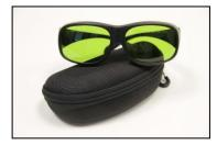
Model: SG-04B Wavelength: 800-1100nm L-rating: 808 – 980nm DIR L5, 1000-1070 DIR L7 Application: 808nm, 980nm laser diode protection, 1064nm YAG laser protection. Transmittance: 60%
