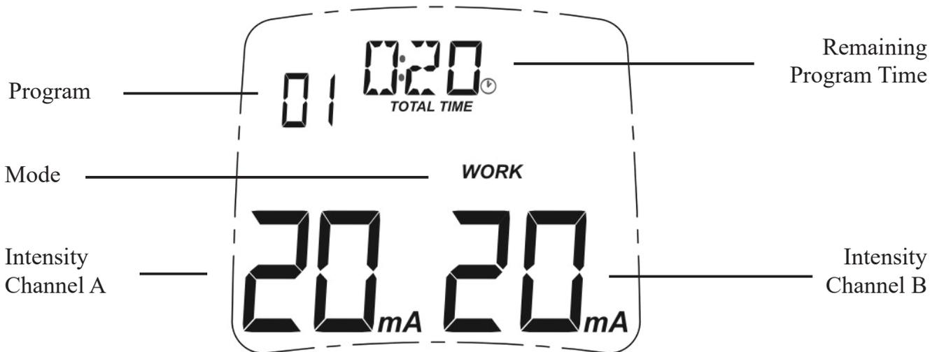
In the upper row you can see the remaining program time and in the bottom line the intensity being applied to each channel. If the button „+” is pressed repeatedly the intensity of stimulation increases. If the button „-” is pressed repeatedly the intensity of stimulation is reduced. For the setting of the intensity it is vital that one feels the electric current but that discomfort never occurs.
