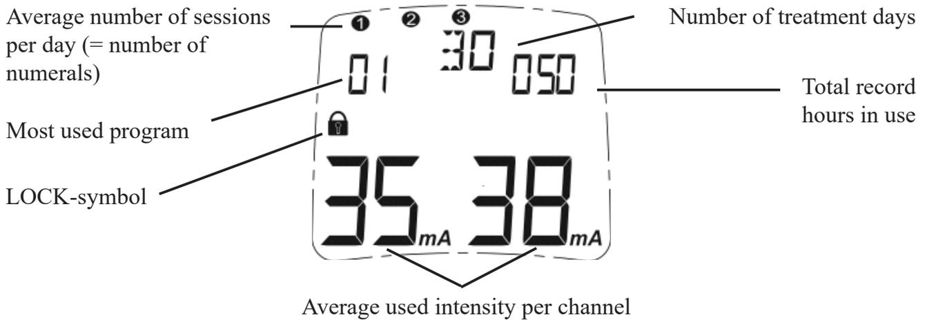
If the program was not locked, it is necessary to press the LOCK button twice to read the memory. The statistics are always recorded regardless of whether the unit is locked or unlocked. The statistics should be reset after 60 days of use or if the device is used by another person.
