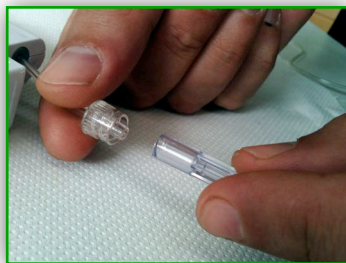
Connection "luer-lock" tube-probe
